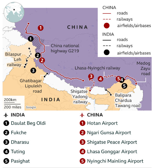
Key infrastructure along India-China border Projects completed or under construction
